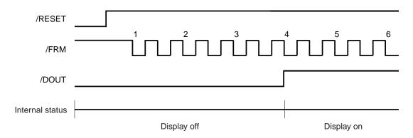
Be sure to initialize the LSI by /RESET when turning on the power.
