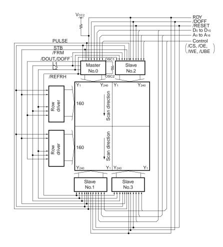
Remark The /DOFF' pin is an input pin of row driver.
