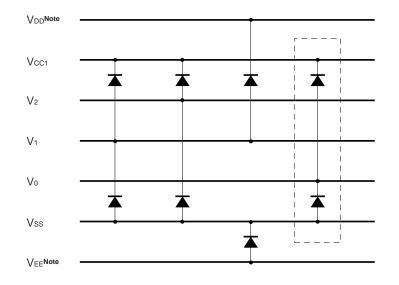
(Use Schottky barrier diodes that are  $V_f = 0.5 V$  or less.)
